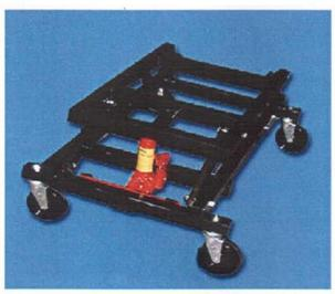
The pool trolley is a device for lifting and moving pool tables with a total weight **no greater than 600kg**. The trolley must only be used on a stable, flat surface and is not designed for external use. For guidance, a standard 7' x 4' coin-operated table with a slate bed would normally weigh in the region of 300kg with the slate and legs fitted but please refer to the table manufacturer for a detailed specification.
